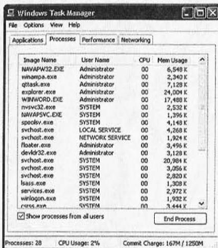
Figure 1: The Windows XP task manager. Users can terminate running programs by selecting them from the list and clicking the "End Process" button.
