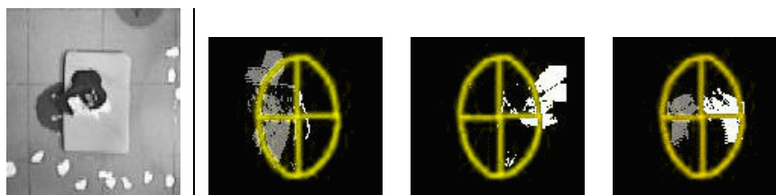
Figure 11: These images show the motion energy that is detected from the overhead camera when a person is “rowing” as they sit on top of the bed. The ellipse represents the position and orientation of the bed, extracted by the system; the colored pixels indicate where the system detected motion. The left, middle, and right images show rowing on the left, right, and both sides of the boat, respectively. The amount of movement at any time is compared with the maximum movement detected so far to compute how vigorously people are rowing and on which side of the bed.
