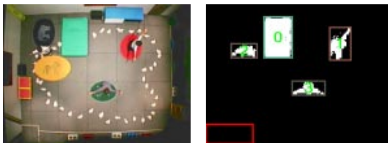
Figure 10: The left image shows a view with three people in the room from the overhead camera used for tracking. The right image shows the output of the tracking system, which is described and evaluated elsewhere [17]. All three people and the bed are being tracked as they move about. The box in the lower left denotes the room’s door region, where all objects must enter and exit. The KidsRoom tracks up to four people and the bed.
