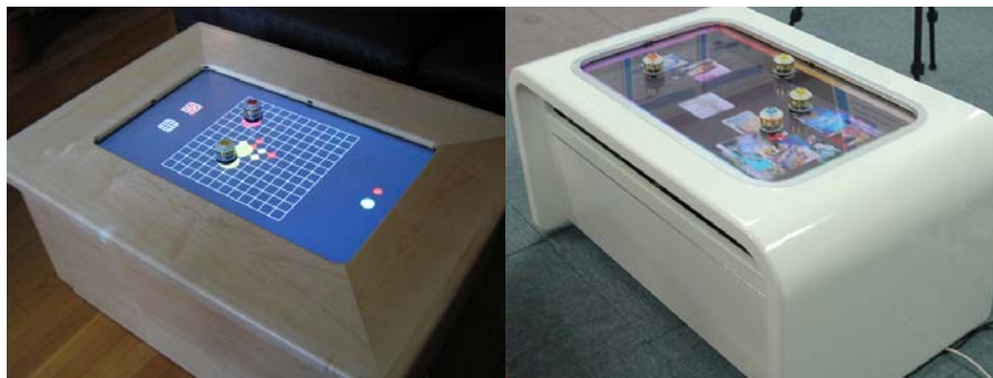
Figure 6: TViews media tables were constructed in two different furniture styles at the MIT Media Lab (left) and Samsung Research (right).
